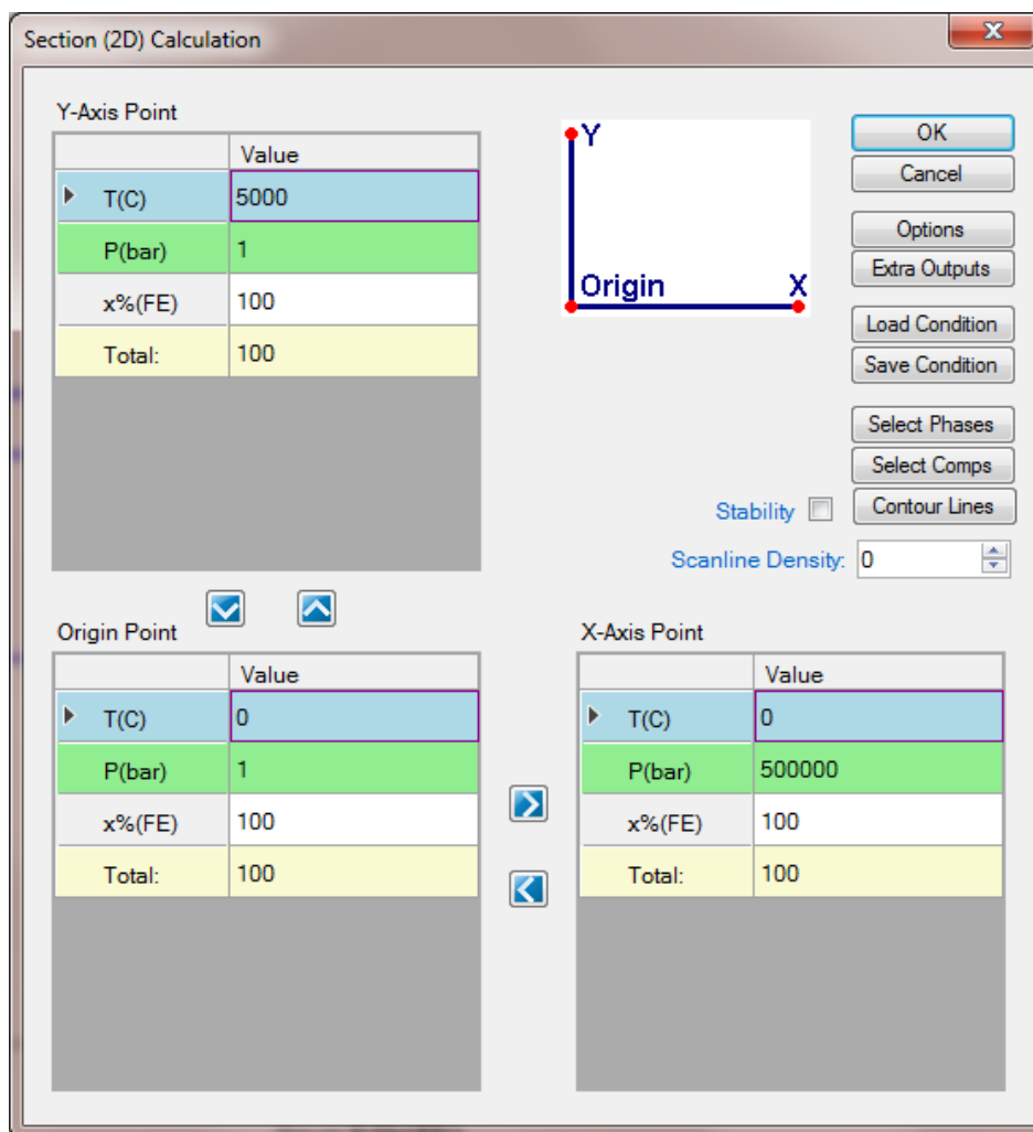
Figure 1.18.1: Setup calculation of T-P diagram for pure Fe, x-axis is P and y-axis is T
